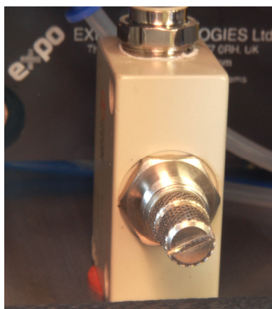
Figure 12. Flow Control Valve (FCV)
