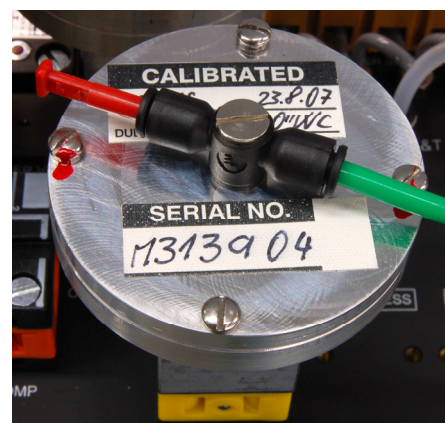
Figure 11. PE or MiniPurge ® system pressure test point
