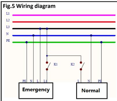
The charging conductor L1 and the luminaire's mains connection must always be connected to the same external conductor of the mains supply!
